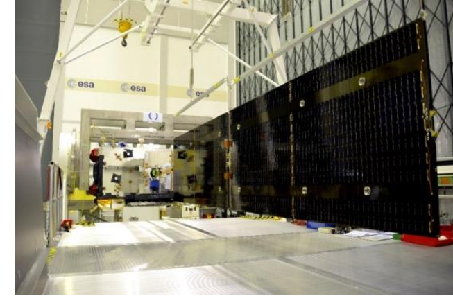
Solar Array deployment test in cleanroom
