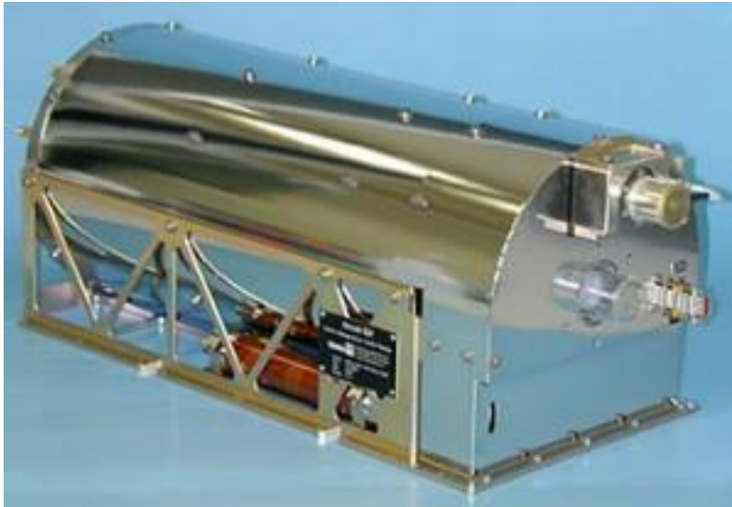
The Passive Hydrogen Maser Clock
